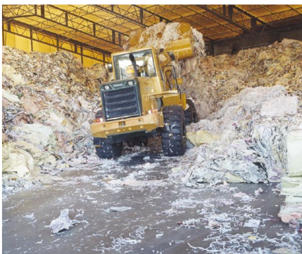
Recovered paper storage area at the Oji Paper Fuji Mill, showing recovered paper being mixed for uniform quality.
