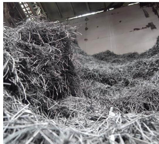
Wires contained in scrap tires. These often cause operational trouble, such as clogged pipes.
