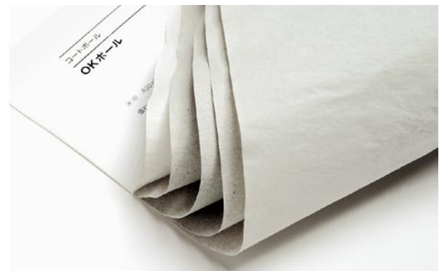
Containerboard and boxboard are structured with multiple layers of thick paper. Each layer uses a different grade of recovered paper.
