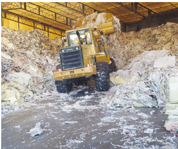
Recovered paper storage area at the Oji Paper Fuji Mill, showing recovered paper being mixed for uniform quality.
