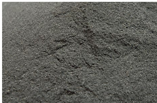
Post-incineration PS ash, which is effectively utilized as a cement and soil enhancer.
